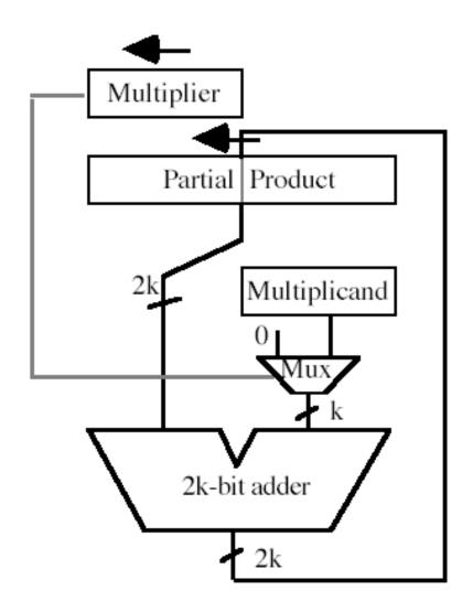
Left shifts are not as efficient for two's complement because must sign extend multiplicand by k bits
