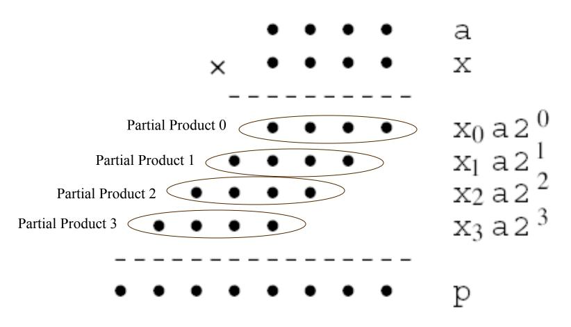
Number of partial products = number of bits in multiplier x Bit-width of each partial product = bit-width of multiplicand a
