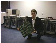
1800 ASIC chips, 40 MHz clock
