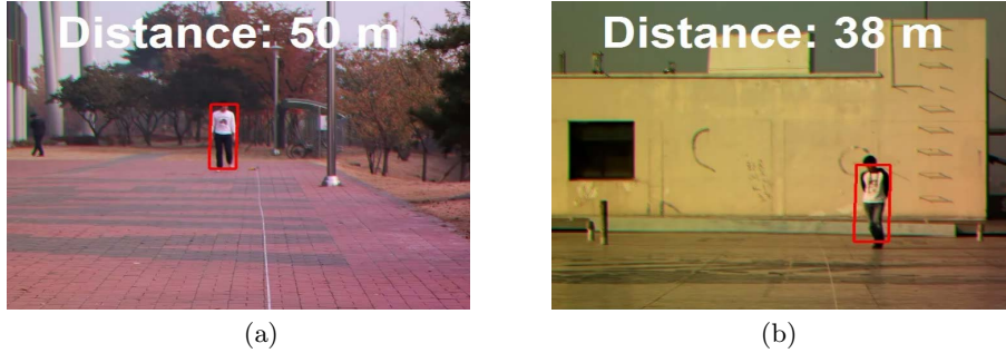
Fig. 7. Frames from a video sequence used to estimate the distance of objects from the camera using a three aperture system
