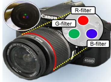
Fig. 1. An SLR camera with three off-axis apertures that are covered by red, green, and blue filters
